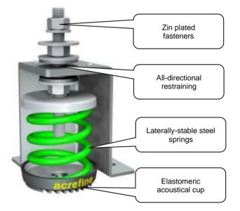
Acrefine ASI-V seismic vibration isolator is designed for floor mounted equipment. This isolator is ideally suited for applications where seismic or high wind forces are likely. Spring deflections of 50 mm (2") provide excellent noise and vibration control.
